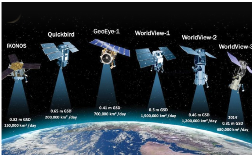
With WorldView-4 joining WorldView-3 in the DigitalGlobe constellation later this year, the total constellation will have the capability to image a location an average of 4.5 times/day at 1m GSD or less
